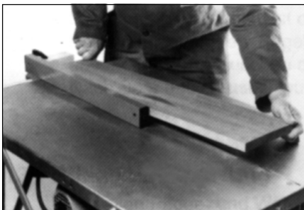
D Important! Mark the area where the saw blade will cut through the work and keep your hands at least 150 mm distance.
